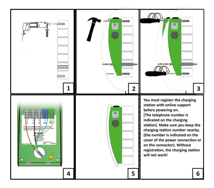
Connect the phase wires<sup>\*</sup> to the indicated L1 / L2 / L3 connecting terminals. Connect the Null wire to the indicated Null terminal. Connect the shield/ground wire to the indicated Ground terminal.
